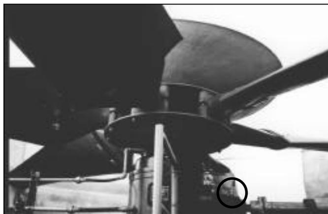
Figures 8, 9 - Permanently mounted accelerometers.
