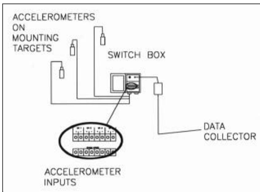
**Figure 7 -** Hardware layout for cooling tower vibration monitoring.
